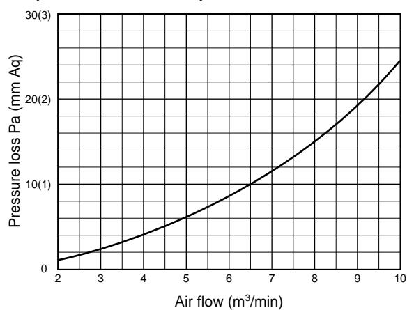
◆ Flexible duct ( $\varnothing 150$ ) friction loss characteristics
