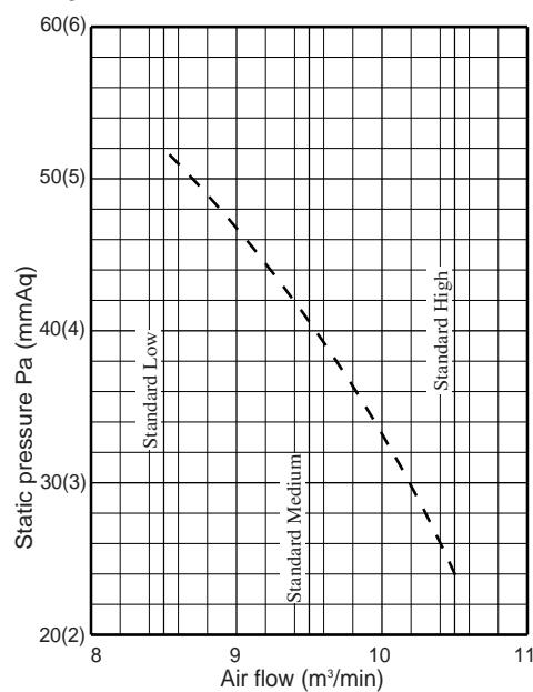
◆ Air outlet unit air flow and friction loss characteristics
