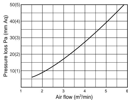
◆ Air inlet grille air flow and friction loss characteristics
